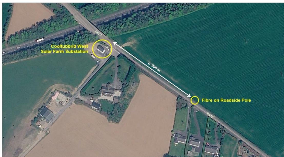
Figure 20. Existing fibre infrastructure on R677 relative to Cooltubbrid Substation
