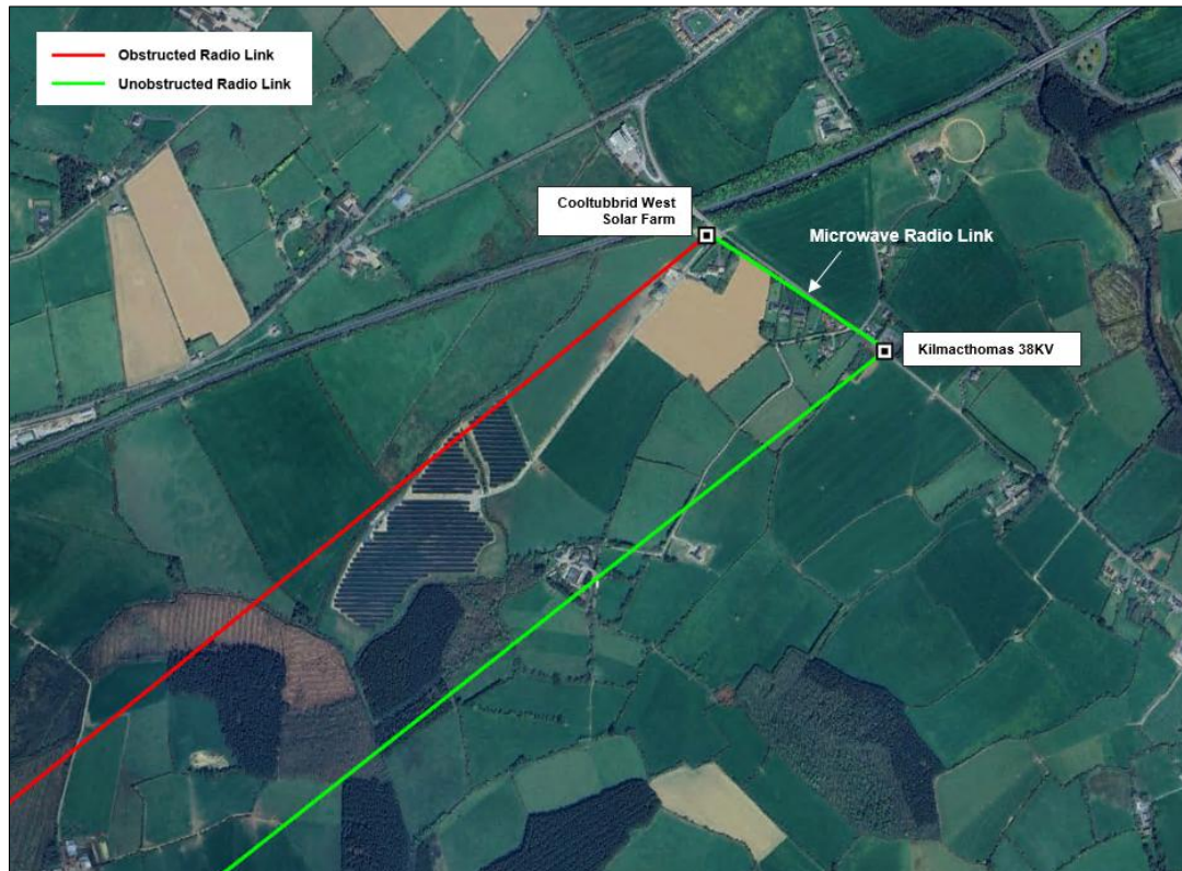
Figure 19. Example of how an existing ESB mast-site could be used to relay the connection between Carrondavderg and Cooltubbrid West Solar Farm.
